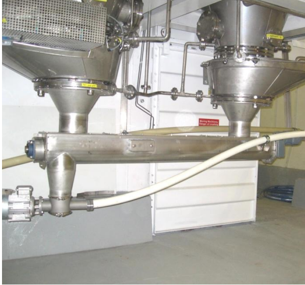
Horizontal trough screw with twin inlets. A flexible screw conveyor is connected to the outlet.
