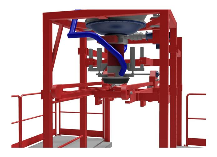
The movable bag suspension yoke moves between three positions: **rigging, filling and automatic unhooking.** Thanks to its mobility and the quick access, it is ergonomic and as such offers and optimum working environment.
