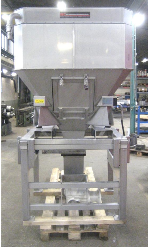
Elevated discharge bowl.
