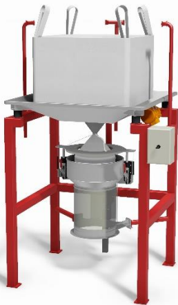
BAGBOY HYGIENE Gen. II type A Floor stand (10a) with bag support (4b) and centering arms (1a). Clamping unit (21) for fixing and stretching the discharge spout, controlled from a pneumatic control cabinet (20).
