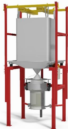
BAGBOY HYGIENE Gen. II type B Floor stand (10b) with bag support (4b), bag suspension stand (1b) and yoke for a fork lift or crane (18c). Clamping unit (21) for fixing and stretching the discharge spout, controlled from a pneumatic control cabinet (20).
