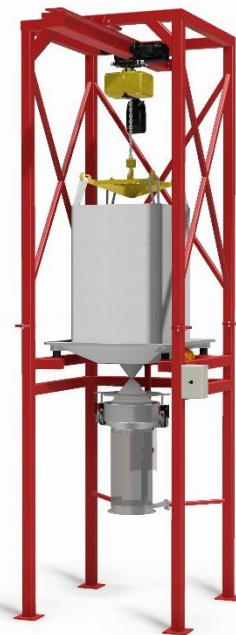
BAGBOY HYGIENE Gen. II type C Crane stand (10c) with bag support (4b), electrically powered chain telpher (17) and lifting yoke (18a). Clamping unit (21) for fixing and stretching the discharge spout, controlled from a pneumatic control cabinet (20).
