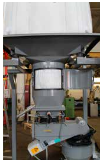
Pneumatic pushers (25) facilitate discharge of material from big bag. Mounted on the stand. Adjustable laterally and vertically.
