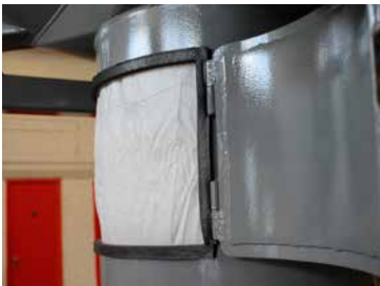
IBC low-profile bag yoke (18b). Includes a counterweight and offers 150 mm negative lift height.
